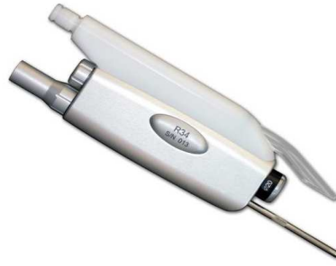
Fig. 3. An example of a 20 mm spot size handpiece (Fotona R34).
