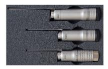
The handpiece can produce 3 mm, 4.5 mm and 6 mm haxagonal spotsizes. Individual spotsizes are selected by simply attaching the optic assemblies marked MIN, MED or MAX (corresponding to 3, 4.5 or 6 mm spot sizes, respectively).
