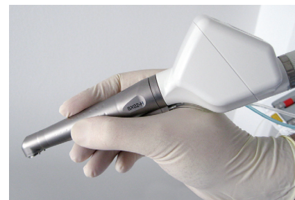
X-Runner, digitally controlled laser handpiece with circular, rectangular (line or square) and hexagonal shape (or shape outline) patterns.
